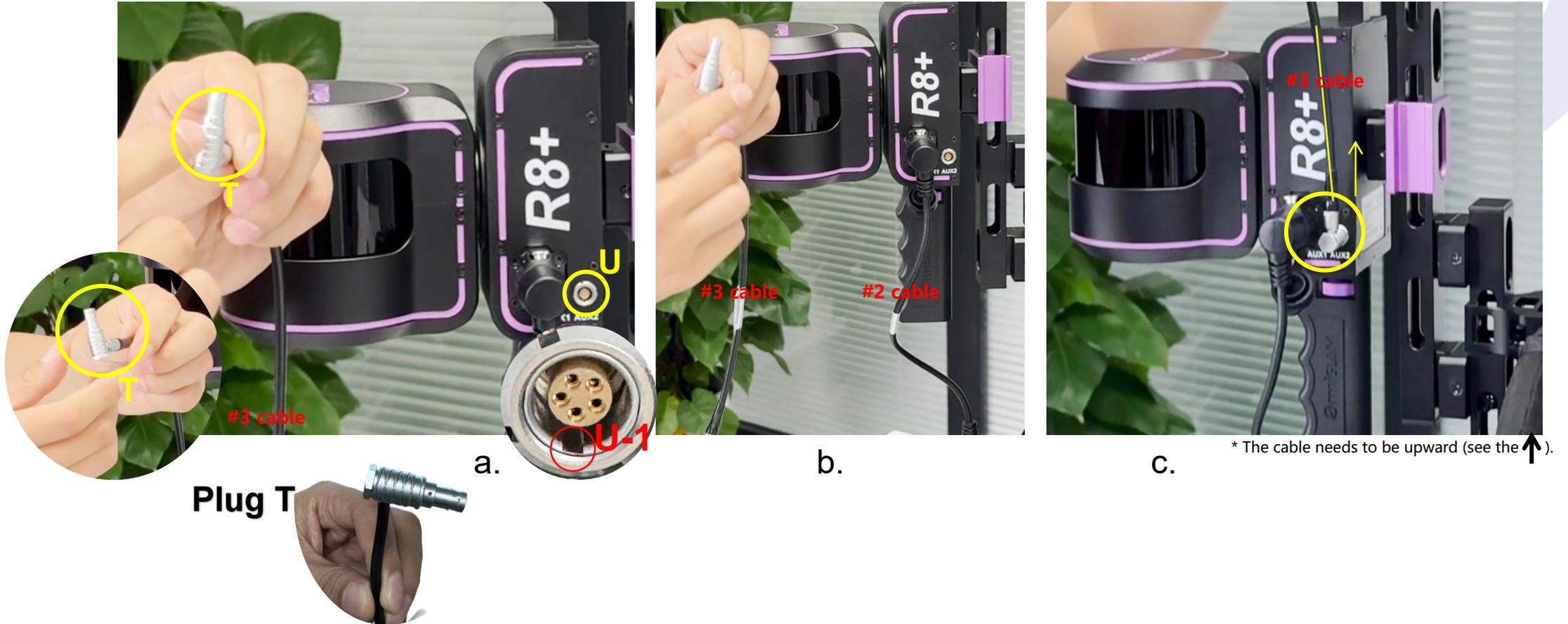
\* The L-shape Plug is for the Handheld Module (interface U).
